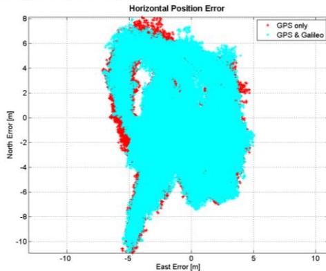
Figure 6: Horizontal Position Error
